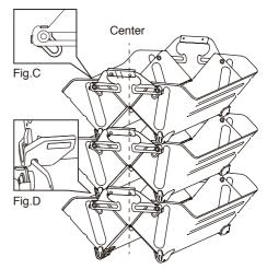
Check that all of the locking pieces are as shown in Fig. C.
